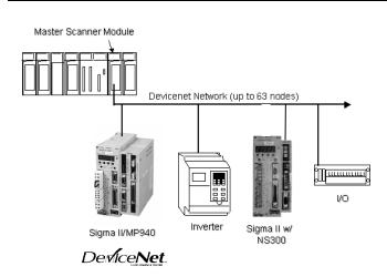
Recent advances in fieldbus increase the flexibility of communications with many different elements of the control system. MP940 allows high performance motion control wider accessibility from cell and process controllers. This simplifies monitoring, set-up and troubleshooting of the machine and process.
