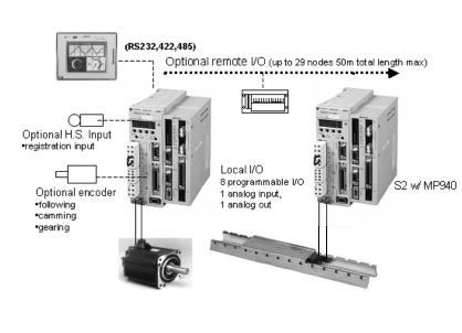
Larger systems link (no additional MP940 hardware requirements) remote I/O modules, and Sigma II/MP940 axes. Up to 8 bytes of input and 8 bytes of output data can be shared with each node in real time with up to 14 MP940 nodes per system. **Multiple servo axes can be synchronized within 2 ms.**
