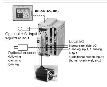
For applications with a fixed amount of I/O requirements, the MP940 includes a rich instruction set of ladder, math, and motion functions with 80kB of memory and 32-bit processing power for several motion programs, conditional logic, fault handling and power-up routines.
